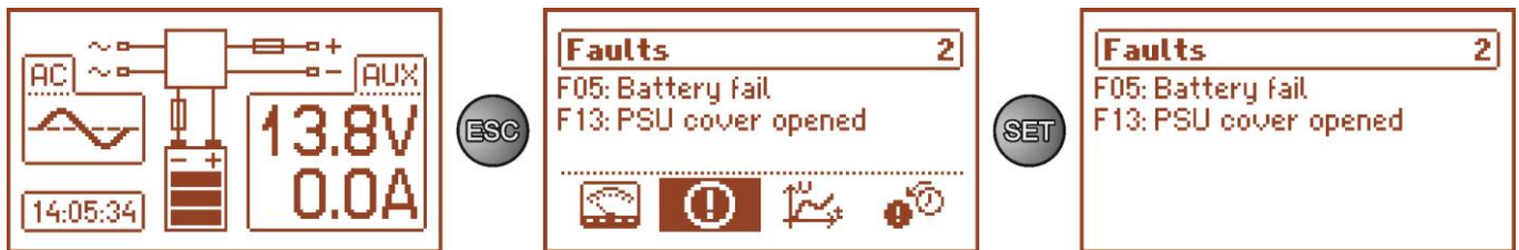
Fig. 10. LCD screen – current failures of the PSU.
